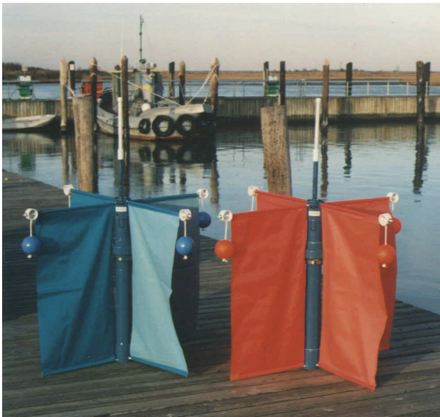
Surface-following Davis/CODE drifter hull, available in two color schemes. High visibility colors help prevent shipstrikes and aid in retrieval, low-visibility colors minimize nuisance pickup of drifters by boaters.
