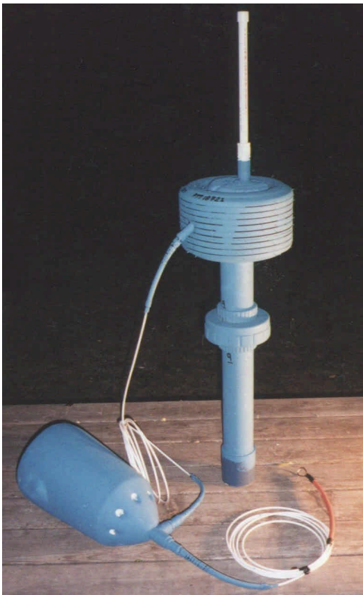
Long duration hull used with deep drogue.
