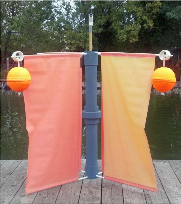
Standard hull with CODE floats and sails attached.
